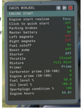
Throttle: Indicates the position of the throttle and if it is set correctly for engine start (1" open)
